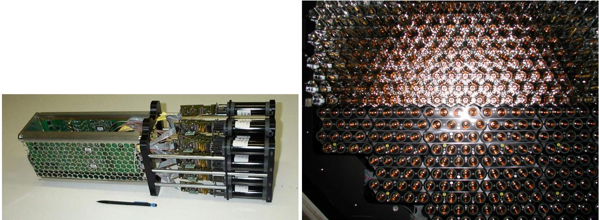
**Figure 3.7:** *Left:* a "drawer", consisting of 16 PMTs and all associated electronics. *Right:* front image of a HESS-I camera. In the upper half the hexagonal Winston cones are already in place, while in the lower half, one can see the bare PMTs. From <https://www.mpi-hd.mpg.de/hfm/HESS/>
