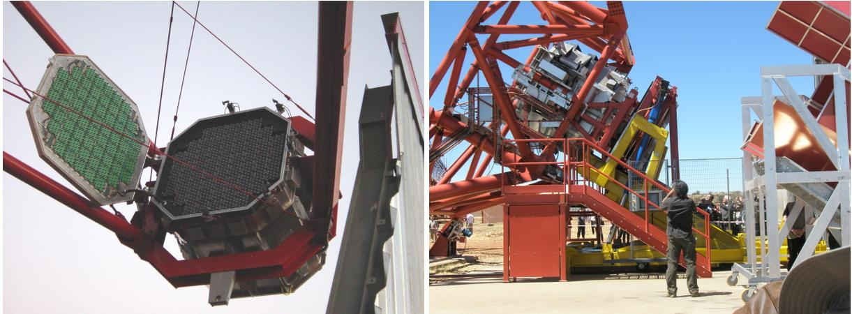
**Figure 3.8:** *Left:* HESS-I camera with open lid inside its support (from <https://www.mpi-hd.mpg.de/hfm/HESS/>). *Right:* CT5 camera being unloaded from the quadrupod as demonstration during the inauguration in September 2012.
