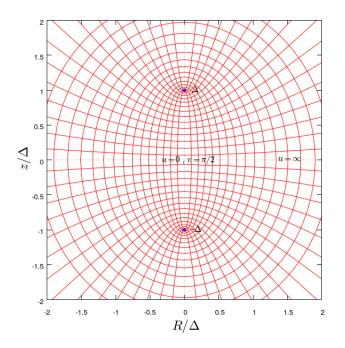
Figure 3.2: Prolate spheroidal coordinate system. Surfaces of constant u are ellipses elongated along the z-axis and surfaces of constant v are hyperbolas.
