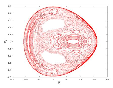
Figure 1.5: Surface of sections using Henon-Heiles potential. We can recognize ordered figures which correspond to regular orbits and are immersed in a 'sea' of irregular orbits.
