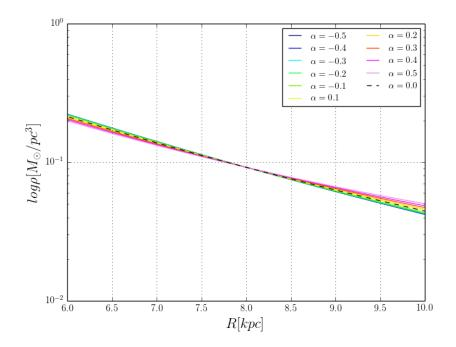
Figure 3.19: Radial density profile for the power-law potential for  $\Delta = 4$  kpc with different values of the power-law index  $\alpha$ [-0.5:0.5]. The dashed line corresponds to the case of  $\alpha = 0$  which corresponds to the logarithmic case.
