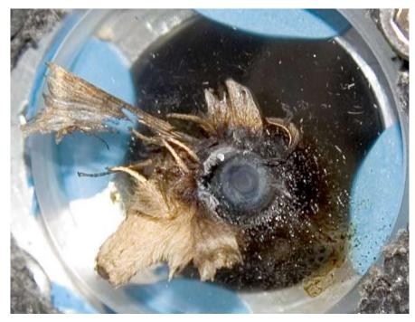
Figure 14: A moth that was killed by the 30W at 523nm laser beam of the MMT, and burned into the surface of an exit window. Image courtesy of MMT.
