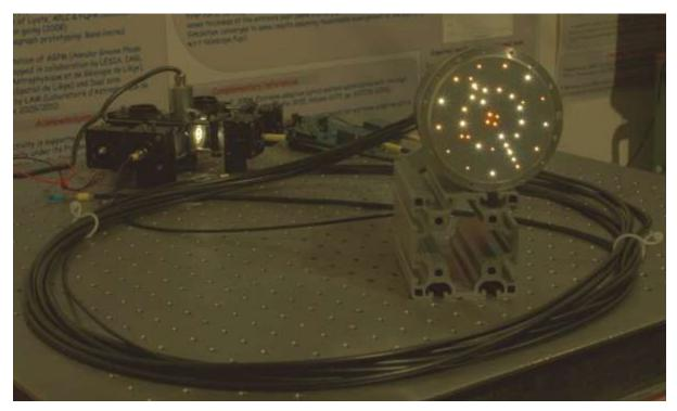
Figure 18: Source module for the GALACSI Calibration Unit. Fibers of different diameters, fed with light of different wavelengths to simulate NGSs and LGSs are precisely arranged in a metal plate. *Picture courtesy ESO*.
