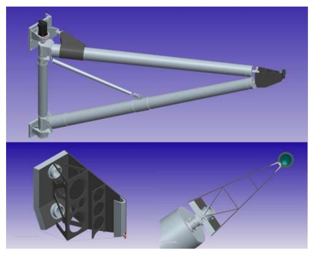
Figure 60: Drawings of the swing arm. Top: The whole arm, ~4.50m long. Bottom: the front end interface, designed to minimize the obstruction of the beam.
