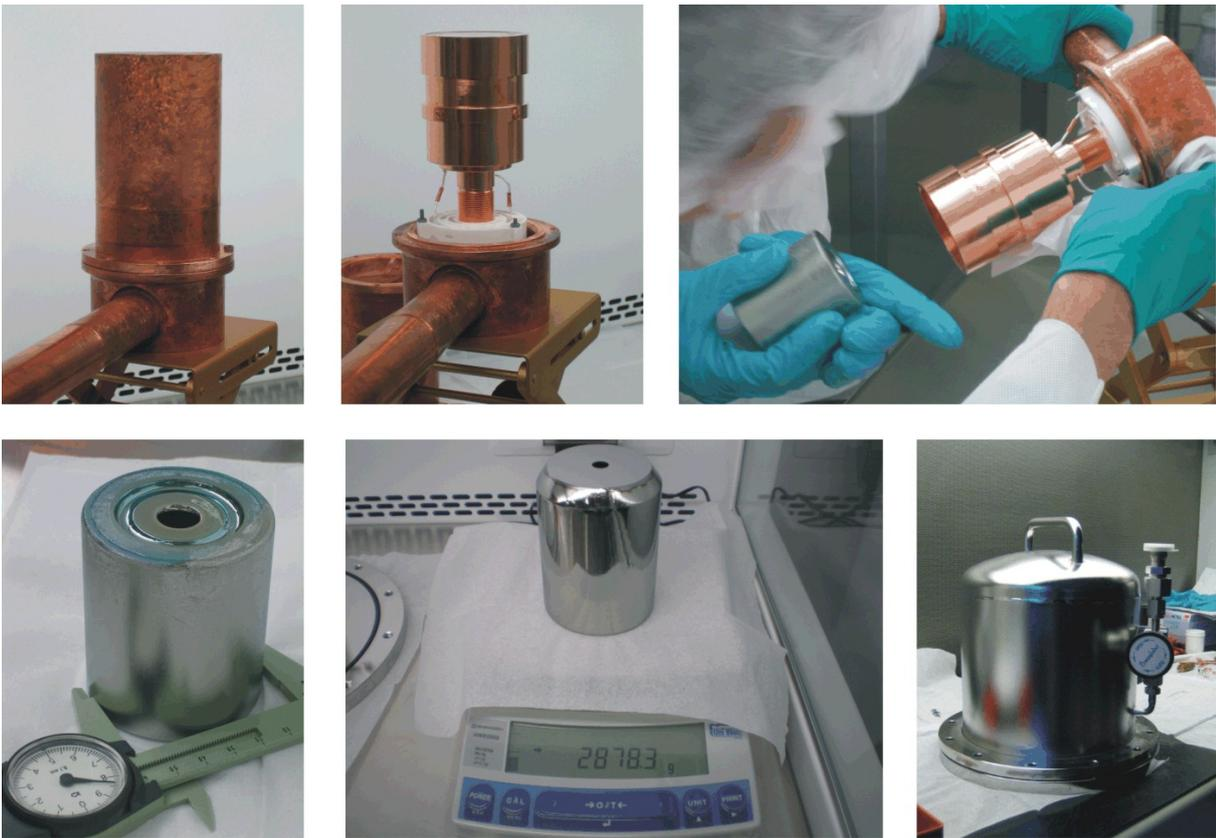
Figure 6.2: Sequence of a diode dismantling and measuring (from top left to bottom right): opening of the cryostat; disassembly of the detector holder; diode taken out from its holder; dimension measurement; mass measurement; storage under vacuum.
