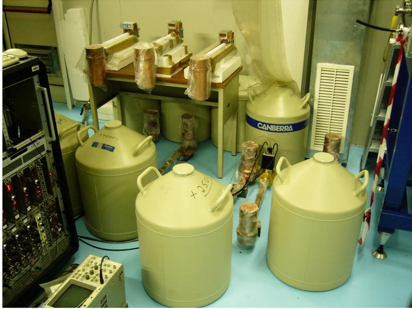
Figure 6.1: Picture of the five Heidelberg-Moscow and three IGEX enriched detectors in the GERDA underground Detector Laboratory, LNGS.
