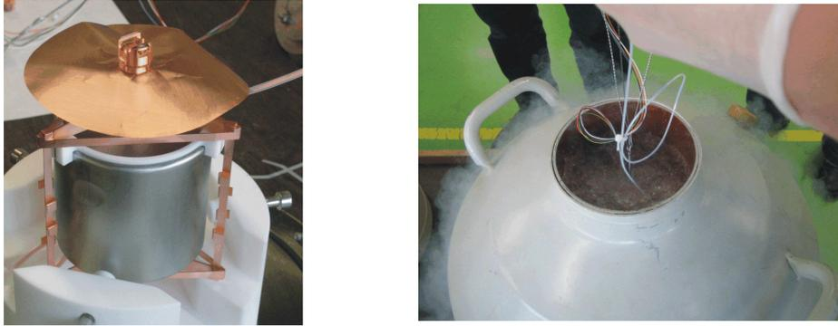
Figure 2.7: **Left:** Infrared shield mounted on top of the prototype assembly. **Right:** Dewar filled with liquid nitrogen in which the detector was operated.
